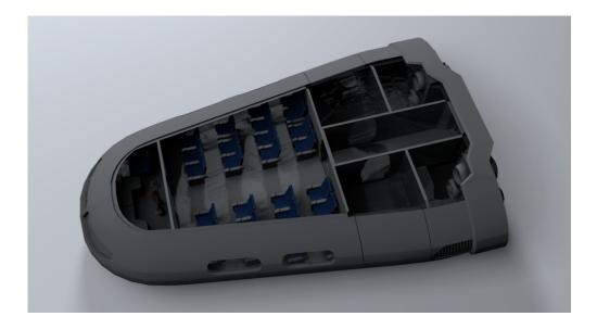
The image above shows a 30 ton Versiil Class Patrol Boat. To imagine the layout of the 20 ton Safari Launch described here imagine the following: The rear portion of the craft is moved forward to the approximate location of the rear cargo bay walls in the image above. The drives would be located at the location of the cargo bays above. The Passenger compartment is nearly the same size and misses the two center rows of seats. The total capacity for the Safari Launch is 20 plus 2 crew.
